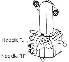
Set the High needle (H) for the highest RPM. After you are satisfied with High-end, adjust the Low (L) needle for smooth transition between High and Low range with out any hesitation.
