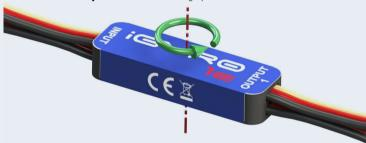
The **iGyro 1e** must therefore be installed in such a way that the device's rotational axis (shown red) lies parallel with the axis of the model which you wish to stabilise.
