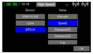
The left-hand column shows all the connected sensors, while the right-hand column shows all the values which these sensors supply. The **P²BUS** is an in-house development, and is capable of transmitting up to 255 sensors each with 32 individual values – and at a speed of up to 800 values per second!
