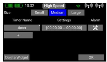
To configure the timer, press the field under **Settings**. The first step is to set the **Start** and **Stop times**: if the **Start time** is greater than the **Stop time**, the timer counts down; if the **Stop time** is greater than the **Start time**, it counts up..
