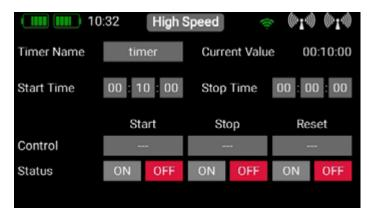
The next step must be to select a **transmitter control** which starts the timer: briefly press the empty field below Start. The **transmitter control** can be a switch, a linear control or a virtual switch. In our example the throttle stick is used to start the timer. Your chosen transmitter control now appears on the left, together with a bar display containing two switching points.
