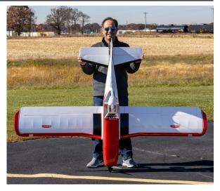
improve slow-speed handling while also offering versatile takeoff and landing abilities. LED landing lights and a clear canopy add to the scale look and flying experience, while tundra-style wheels/tires make it possible to fly from paved, dirt, gravel, and grass surfaces. The factory-applied UltraCote film and painted-fibreglass parts finish saves you time and looks great, plus the two-piece, plug-in wing makes it easy to transport and store.
